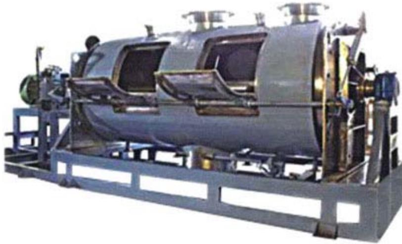
S.S Engineering Plough Shear Mixer has a horizontal cylindrical shape with flat end plates. The main shaft passes through the axis of the vessel and is supported at the end plates in specially designed bearing housing. The plough shaped mixing elements are arranged concentrically on the main shaft. The clearance between the ploughs and shell wall is minimum, to facilitate better mixing.
